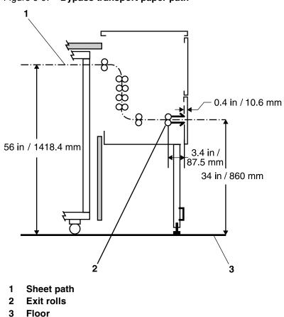
Figure 6-9. Bypass transport paper path
